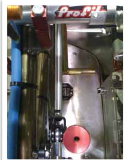
TOP VIEW FRAME, MASTER CYLINDER RODS BRAKE ROD ALL RUNNING PARALLEL
